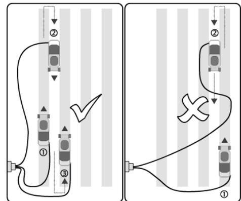
**Warning:** Do not mow towards the cable as shown in right picture.
