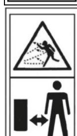
Risk of ejection. Keep unauthorised persons away from the work area while the machine is in use.
