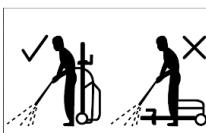
The high pressure cleaner must be used on a secure and stable surface in a standing, upright position.
